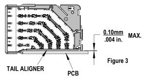
There should be no broken stand-offs along the perimeter of the part (an indication of over-pressing).
