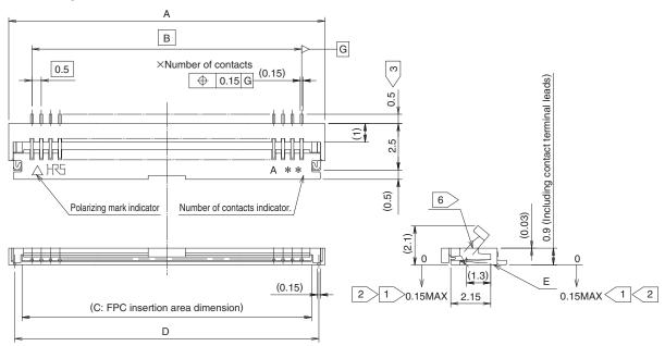
Notes 1 The coplanarity of each terminal lead and metal fitting is within 0.1
