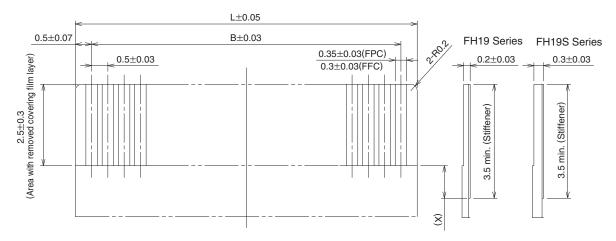
Note1: Polyamide and a thermally hardened adhesive is recommended as the materials for the stiffener.
