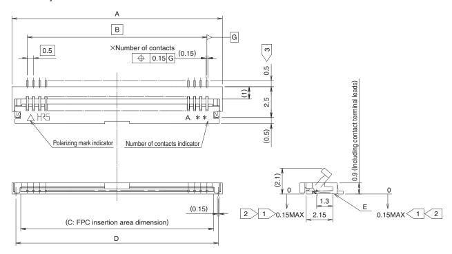
Notes  $\boxed{1}$  The coplanarity of each terminal lead and metal fitting is within 0.1
