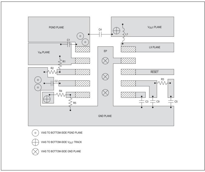
Figure 4. Recommended Component Placement for MAX17542G
