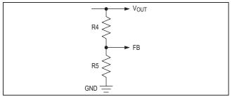
Figure 1. Setting the Output Voltage
