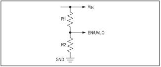
Figure 2. Adjustable EN/UVLO Network
